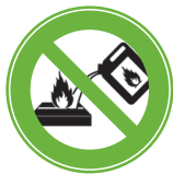
Do not fill while operating
