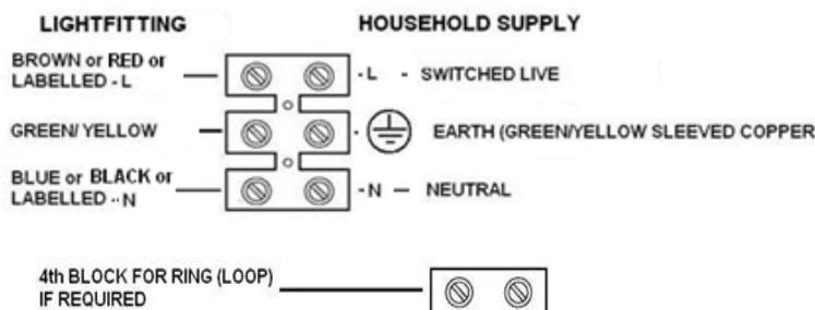
1. Decide on the position of the light fitting / or remove existing light fitting. Take a note of the position of the electrical connections. Ensure there is a solid mounting surface, preferably a wooden joist or joist bridge to support the weight of the light fitting.
