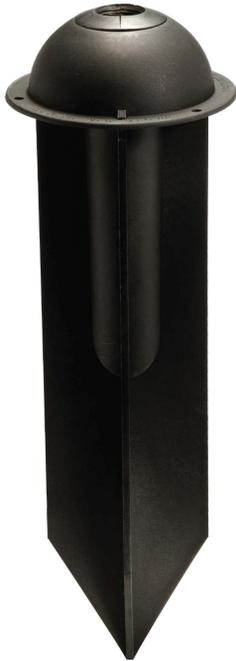
The Hunza Super Spike 25mm is a multi purpose ground spike which adds significant stability when used. It is designed for use with Hunza luminaires that have a 25mm diameter pole or 1/2" NPS thread. It is supplied with two snap in adaptors and is constructed from UV black polycarbonate. There is sufficient space for a cable connection under the dome. It is suitable for use with aluminium, copper and 316 stainless steel luminaires.
