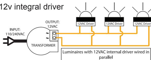
Luminaires with 12VAC internal driver wired in parallel
