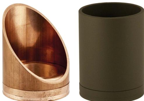
The Glare Guard serves two purposes. Firstly to protect the eye from the direct glare or the sparkle effect from the lamp and secondly to guard against any direct light which may be emitted from the lens of the fitting. An additional lens can be fitted to keep the luminaire free of debris being deposited in the glare guard.
