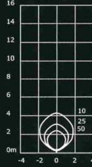
100 watt Mini White Son IR Filters Fitted 24° Beam GX12.1 5000 Lumens I-Max = 13120 cd
