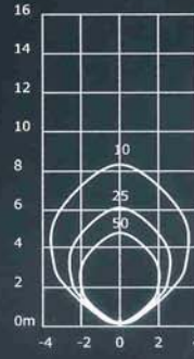
150 watt Metal Halide 60° Beam G12 14000 Lumens I-Max = 11820 cd
