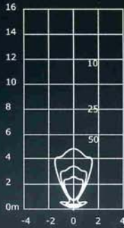
60 watt IRC Halogen 45° Beam G53 1400 Lumens I-Max = 2790 cd
