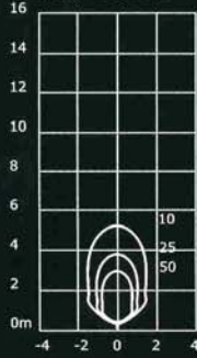
100 watt Mini White Son IR Filters Fitted 12° Beam GX12.1 5000 Lumens I-Max = 58750 cd
