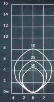
150 watt Metal Halide IR Filters Fitted 60° Beam G12 14000 Lumens I-Max = 10640 cd
