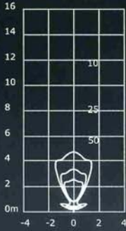
60 watt IRC Halogen IR Filters Fitted 45° Beam G53 1400 Lumens I-Max = 2500 cd
