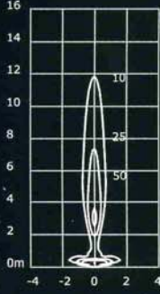
60 watt IRC Halogen 45° Beam G53 1400 Lumens I-Max = 2790 cd
