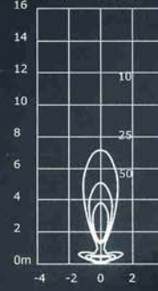
60 watt IRC Halogen IR Filters Fitted 24° Beam G53 1400 Lumens I-Max = 7630 cd
