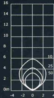
35 watt Metal Halide 24° Beam G12 3300 Lumens I-Max = 9583 cd
