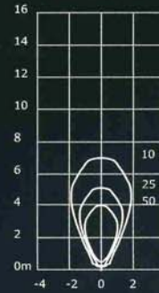
60 watt IRC Halogen IR Filters Fitted 24° Beam G53 1400 Lumens I-Max = 7630 cd
