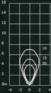
70 watt Metal Halide IR Filters Fitted 24° Beam GX 8.5 6400 Lumens I-Max = 15360 cd
