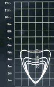
35 watt Metal Halide IR Filters Fitted 60° Beam PGJ5 3000 Lumens I-Max = 1600 cd
