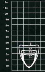
20 watt Metal Halide IR Filters Fitted 60° Beam PGJ5 1650 Lumens I-Max = 1045 cd
