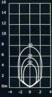
150 watt Metal Halide 12° Beam G12 14000 Lumens I-Max = 182700 cd
