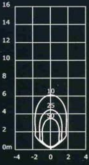
70 watt Metal Halide 12° Beam G12 6600 Lumens I-Max = 86150 cd
