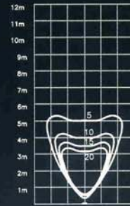
35 watt Metal Halide 60° Beam PGJ5 3000 Lumens I-Max = 1780 cd
