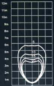
35 watt Metal Halide Asymmetric Lens 60° Beam PGJ5 3000 Lumens I-Max = 1191 cd I-Max @ Zenith -27.50
