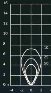
60 watt IRC Halogen 24° Beam G53 1400 Lumens I-Max = 8480 cd
