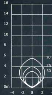
35 watt Metal Halide IR Filters Fitted 24° Beam G12 3300 Lumens I-Max = 8624 cd
