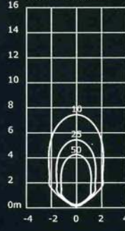
150 watt Metal Halide IR Filters Fitted 12° Beam G12 14000 Lumens I-Max = 164400 cd
