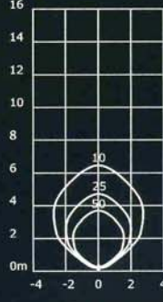
150 watt Metal Halide 24° Beam G12 14000 Lumens I-Max = 40650 cd
