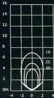
35 watt Metal Halide 12° Beam G12 3300 Lumens I-Max = 43078 cd
