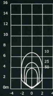
35 watt Metal Halide IR Filters Fitted 12° Beam G12 3300 Lumens I-Max = 38809 cd
