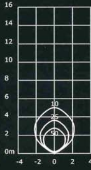
70 watt Metal Halide 24° Beam G12 6600 Lumens I-Max = 19166 cd
