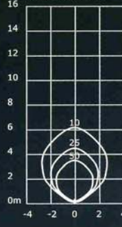
150 watt Metal Halide IR Filters Fitted 24° Beam G12 14000 Lumens I-Max = 36580 cd
