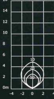
70 watt Metal Halide IR Filters Fitted 24° Beam G12 3300 Lumens I-Max = 17250 cd
