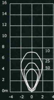
70 watt Metal Halide 24° Beam GX 8.5 6400 Lumens I-Max = 17068 cd
