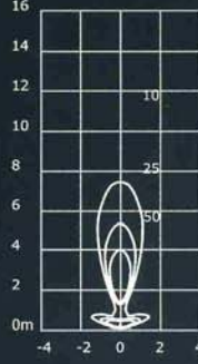
60 watt IRC Halogen 24° Beam G53 1400 Lumens I-Max = 8480 cd
