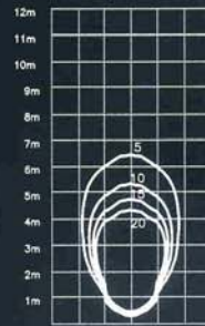
35 watt Metal Halide IR Filters Fitted Asymmetric Lens 36° Beam PGJ5 3000 Lumens I-Max = 3560 cd I-Max @ Zenith -32.50
